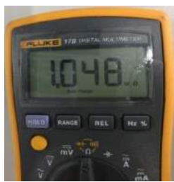
Figure 5-4.6: Measuring resistances among compressor terminals
