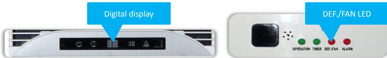
Figure 4-1.3: Indoor unit digital displays and LED indicators
