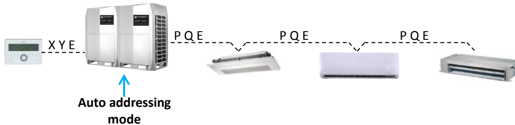
Figure 4-1.4: Indoor centralized controller connected to master outdoor unit
