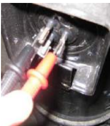
Figure 5-4.6: Measuring resistances among compressor terminals
