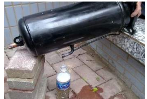
Figure 5-4.14: Draining oil from a compressor
