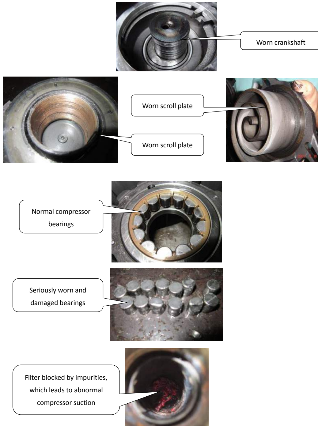
Figure 5-4.17: Effects of spoiled compressor oil
