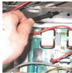
Figure 5-4.7: Measuring resistances between compressor terminals and ground
